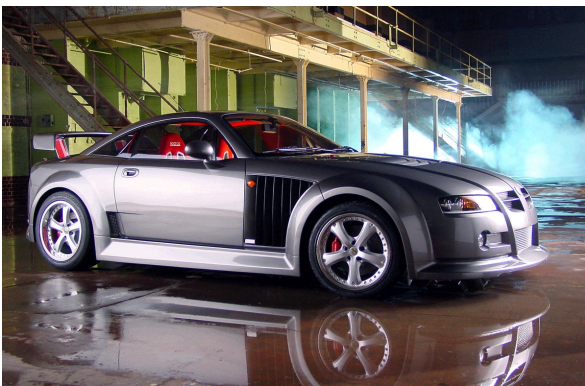
Figure 2: MG Rover X-power SV contains 36 carbon composite components. Structural parts are autoclave cured, while body panels use a vacuum-cured "semi-preg" system.
