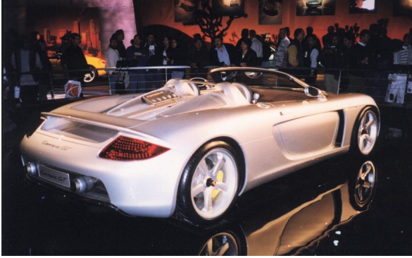
Figure 1: The Porsche Carrera GT is highly carbon-intensive, with body panels and structure produced from autoclave-cured epoxy prepreg.
