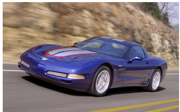
Figure 6: Chevrolet Corvette Z06 Commemorative Edition vehicles will carry an autoclave-cured carbon fiber hood in 2004, the first use of exterior Class A carbon on a North American mainstream vehicle.
