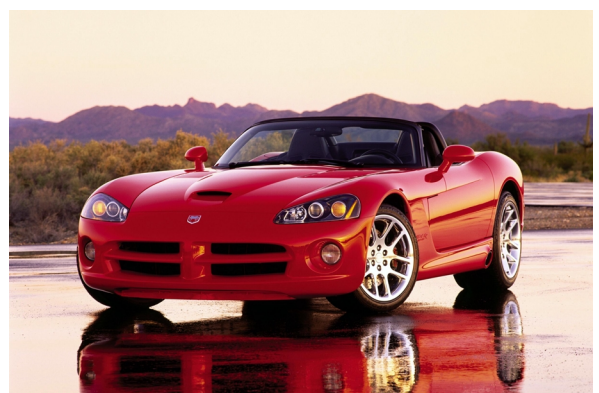
Figure 5: The Dodge Viper SRT-10 marks the first production use of carbon fiber SMC, using the material in the front end structure, windshield surround and door inner panels.
