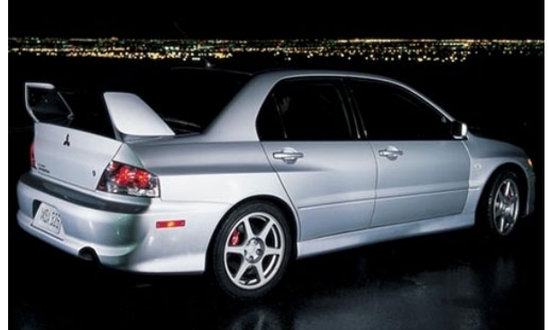
Figure 4: Optional carbon fiber rear spoiler on the Mitsubishi Lancer Evolution VIII is produced via RTM
