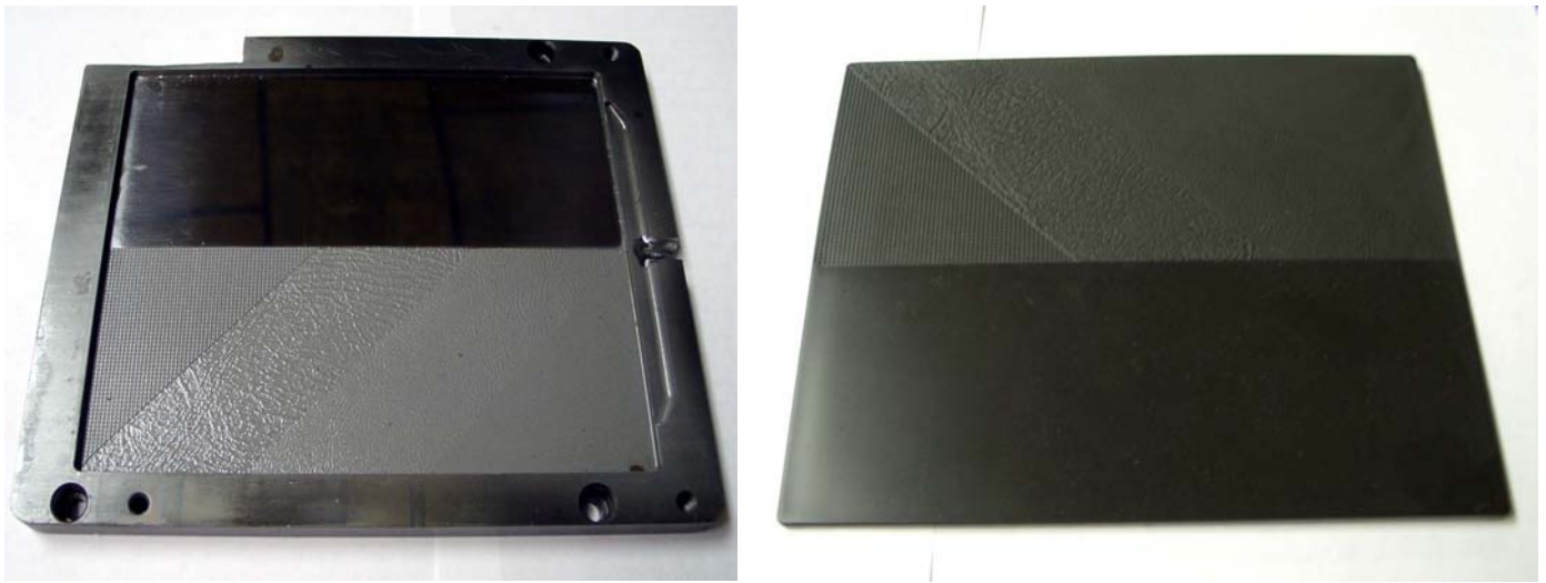
Figure 8. PX-5 Textured Plaque Tool and Injection Molded Polypropylene Sample.
