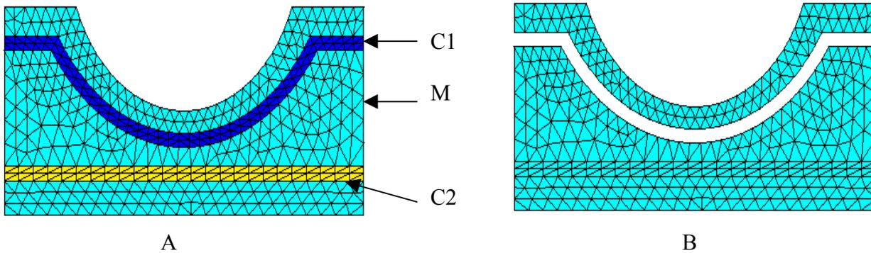
**Figure 3:** Part of the mold with multiple domains. A) The mesh input to the analysis tool is made of domains M, C1, and C2. Any or all can be used for obtaining a solution. B) The mesh obtained out of the union of M and C2 is used for the analysis. This domain is assigned steel as the material type. A convection boundary condition is specified on the exterior of C1 and the mesh in C1 is not included for obtaining a solution.
