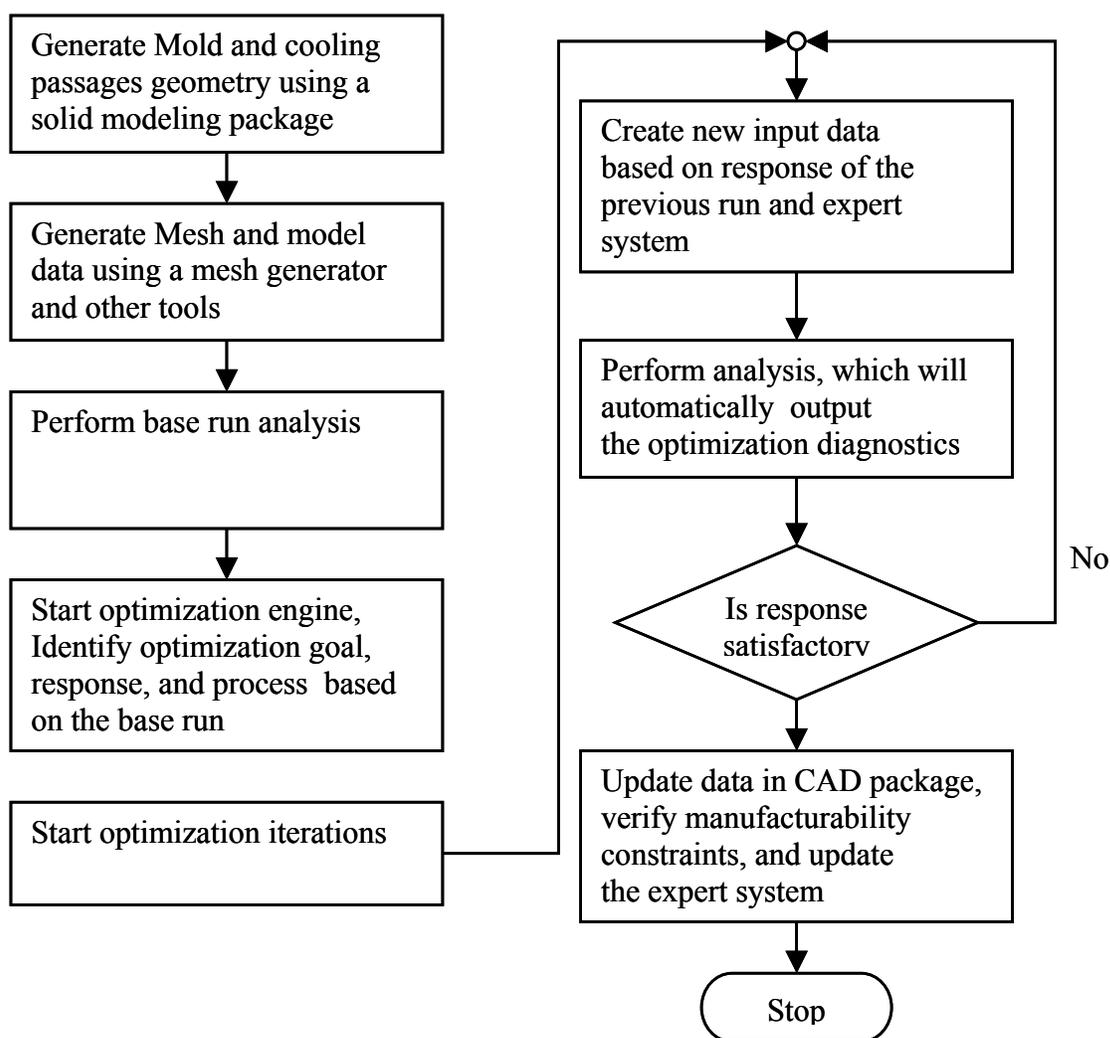
**Figure 2:** Optimization algorithm used to obtain solution
