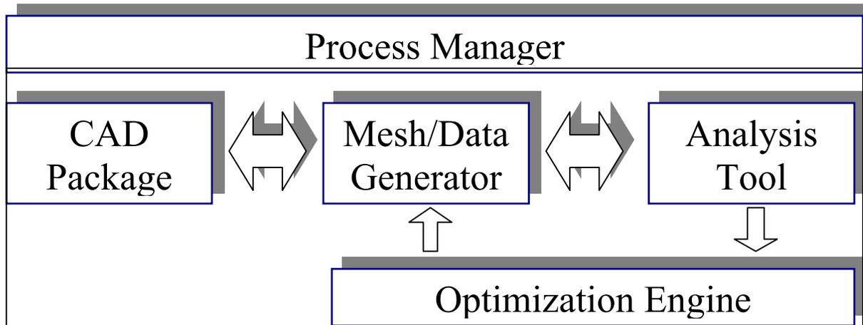
**Figure 1:** Interaction between different tools that are used for simulation. Communication is handled using the Tcl API interface.
