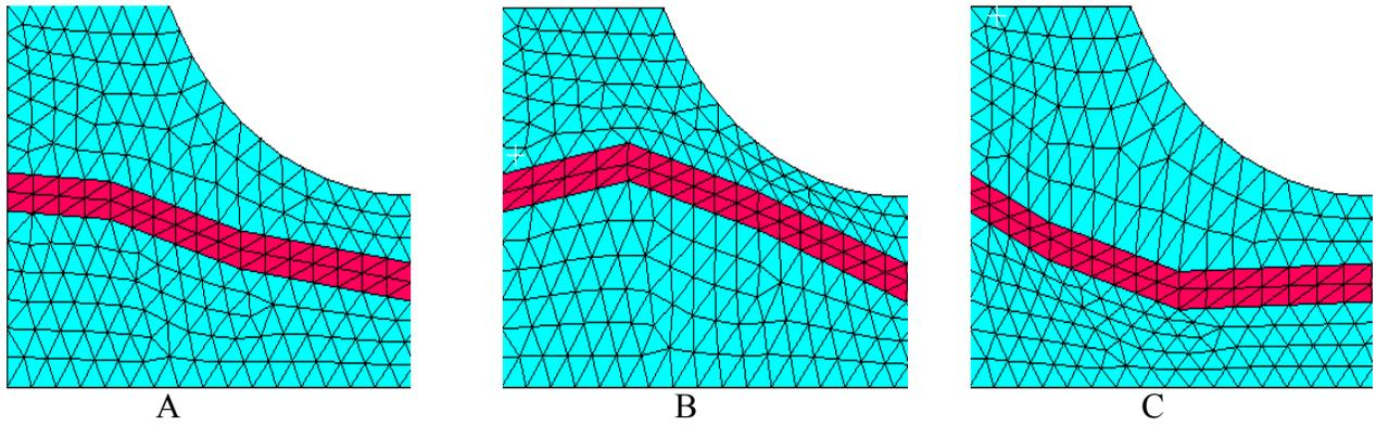
**Figure 5:** The mesh is moved using shape variables generated by Altair HyperMorph®. A) Undeformed configuration, with the cooling channel shown in red. B) Snapshot of a deformed configuration based on a single shape variable. C) Snapshot of a deformed configuration on the other extreme based on the same shape variable.
