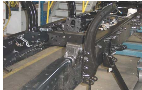
Figure 2: Representative chassis assembly for a Class 8 truck showing a variety of steel members bolted together.
