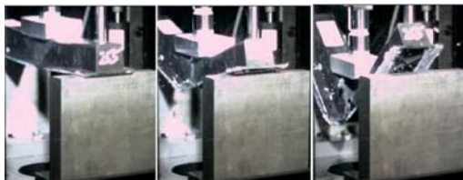
Figure 15: Impact of hybrid bonded using BETAMATE LESA 74020 adhesive
