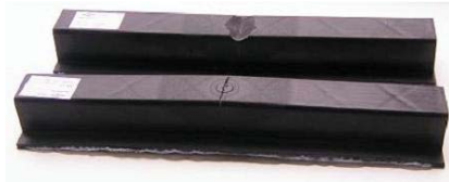
Figure 6: Parts after static bending test
