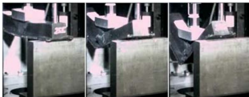
Figure 14: Impact of hybrid bonded with BETAMATE 2810 PU adhesive
