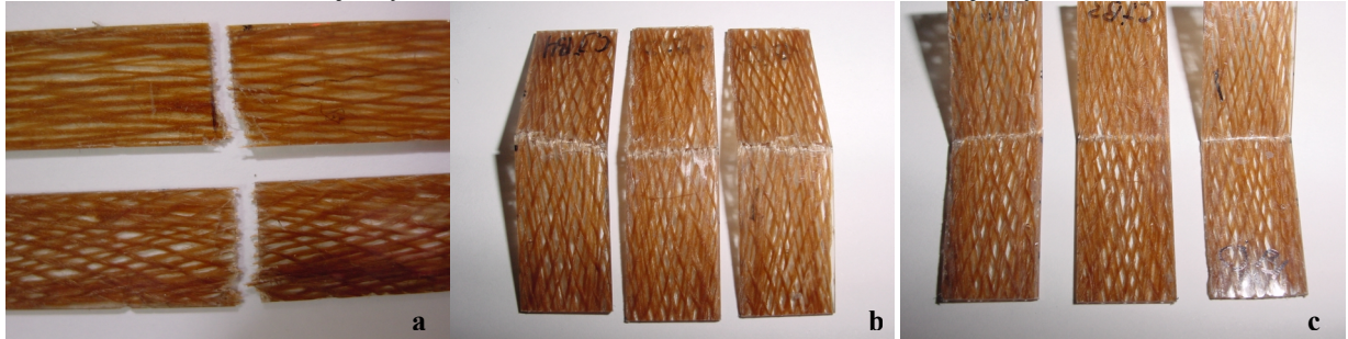
Figure 4: Fractured test specimens (a) Tensile specimens (b) Tension side of Bending (c) Compression side of bending
