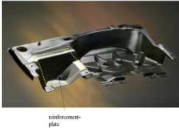
Figure 7: Underbody shield with self-reinforced PP impact and abrasion patch
