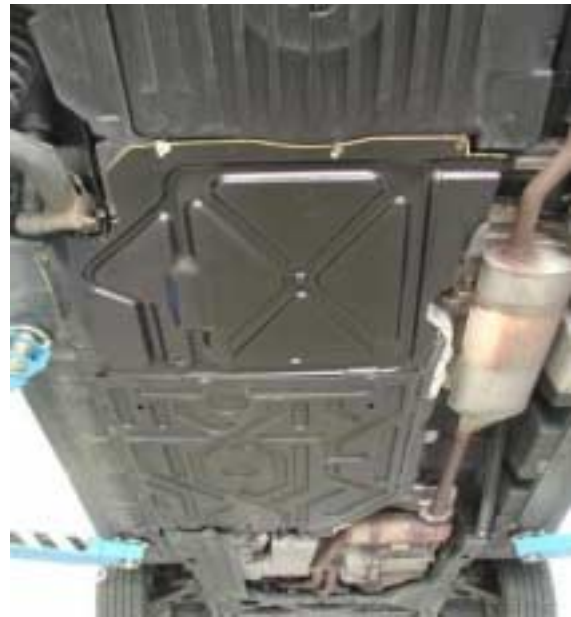
Figure 5: Self-reinforced PP underbody shield (center)
