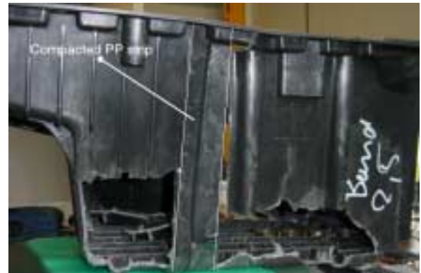
Figure 6: LFT battery box with self-reinforced PP reinforcement strip
