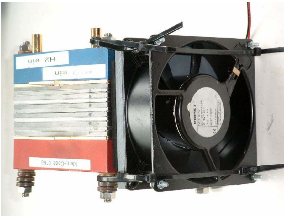
Figure 2. The assembled four-cell stack with fan for forcing air.
