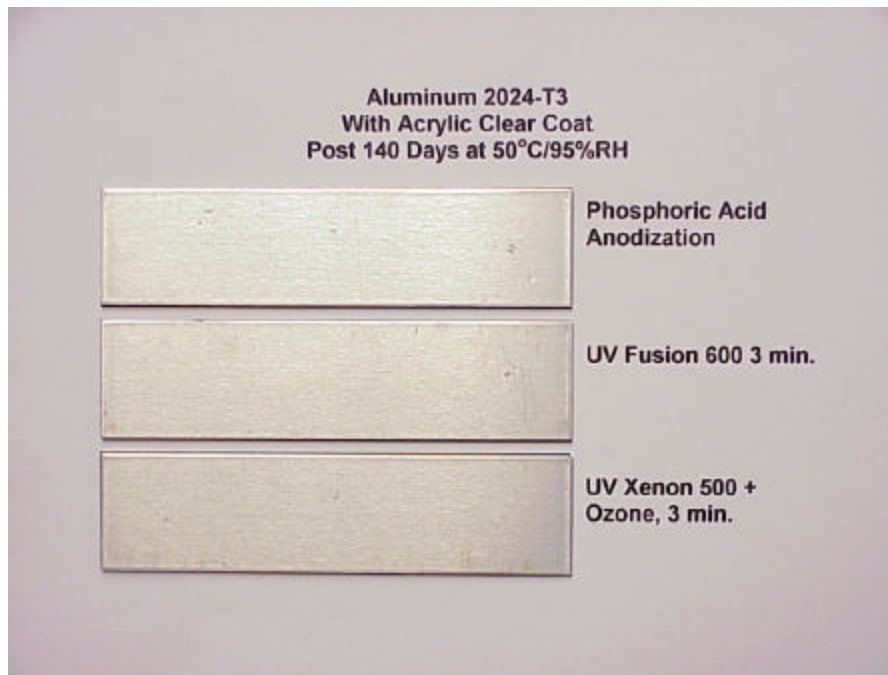
Figure 5. Painted 2024-T3 surface treated with UV or phosphoric acid anodization following humidity conditioning.
