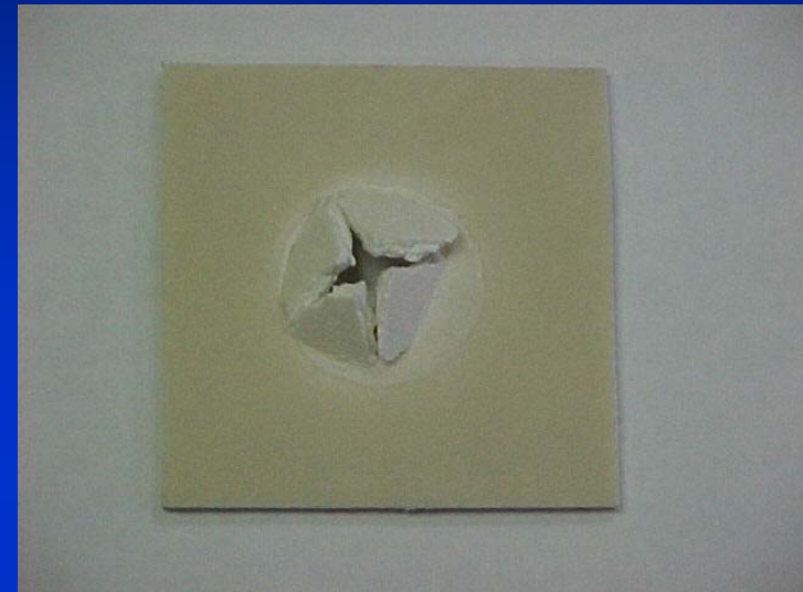
LFT PPGF40 with 5% flame retardant
