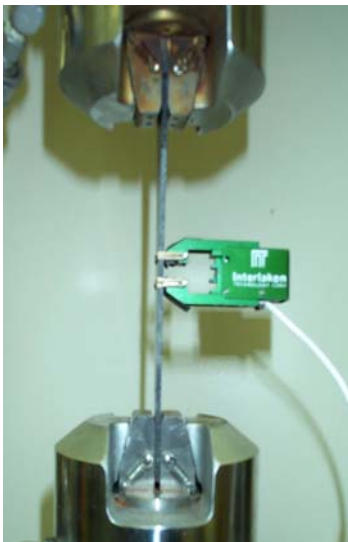
Figure 5. Room temperature tensile test set-up with extensometer for fatigue pre-test profile.
