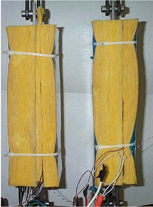
Figure 12. Elevated temperature insulation for tensile creep tests with heaters in place.
