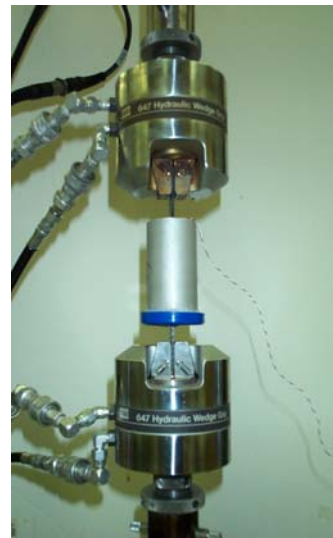
Figure 6. Wet tensile fatigue test set-up.
