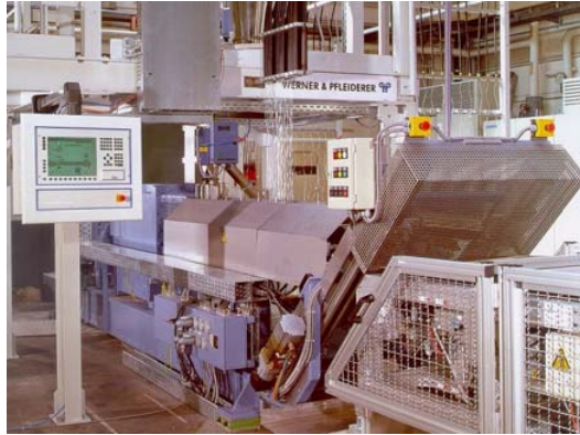
Figure 7: The glass fibers taken off roving bobbin are drawn into the barrel of the twin screw extruder
