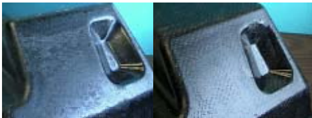
Figure 10. Surface porosity on parts molded with commingled PP/glass mats (left) and twill 2x2 fabrics (right)
