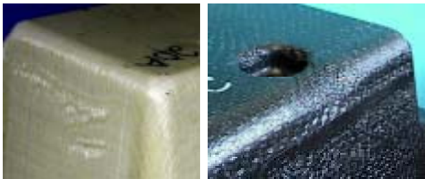
A) B) Figure 9. A) Fibre compression and buckling and B) Fibre compaction and resin percolation along edges and corners.
