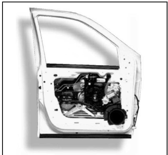
Figure 2, Example of door module fitted in metal door.
