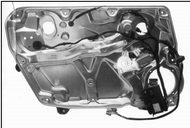
Figure 4, VW Passat sheet metal door module (Brose).
