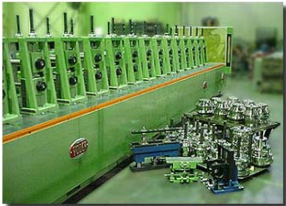
Figure 1. A typical roll forming line.
