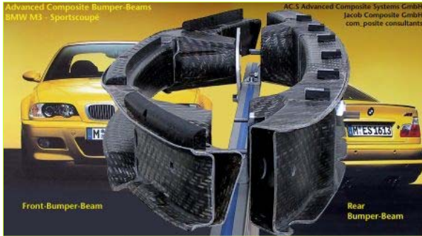
Figure 7. The BMW M3 bumper beam system [3].
