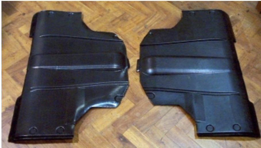
Figure 5. Self-reinforced PP (left) and GMT (right) undershields
