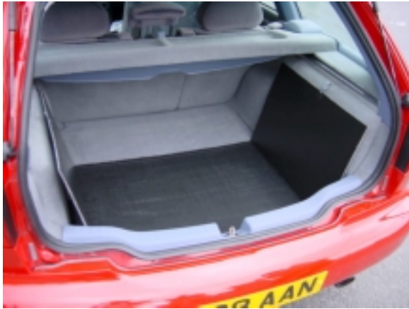
Figure 6a. Self-reinforced PP/honeycomb laminate load floor with carpets folded back to reveal an easy-clean surface
